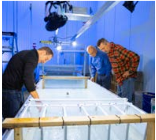
Sean Bennett, PhD (Professor, Department of Geography and Associate Dean, College of Arts and Sciences) and his colleagues use an overhead video camera and an object-detection model to track the shiners' movements, as well as the water velocity, inside the flume. Photo: Douglas Levere
