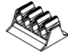
THE CABLE GRIP IS SIMPLY SCREWED TO THE SURFACE WITH FOUR WOOD SCREWS AND THE WIRES SIMPLY SNAP INTO THE STORAGE POSITION BETWEEN THE LOOPS
