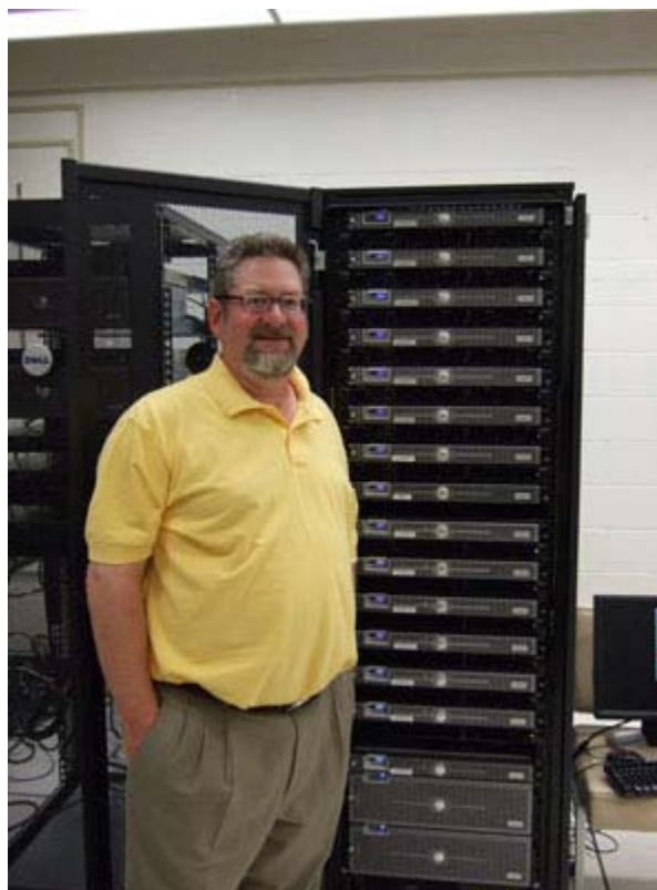
Russ Miller, principal investigator at CI Lab, stands in front of the server rack that holds Magic, a synchronous supercomputer that can achieve up to 50 Teraflops. Image courtesy of CI Lab.
