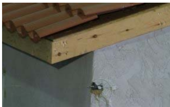
Sensors mounted inside and outside the home gave scientists information about how much the house moved and flexed during the simulated earthquake.
