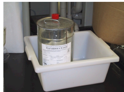
Example of Secondary Containment - Note properly labeled container
