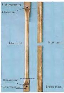
A common approach to measure toughness (ductility) is to pull on the material and measure how far it stretches before it deforms.
