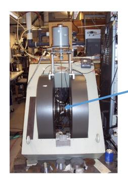
Place magnet inside. Apply different magnetic fields, and measure magnetic flux density
