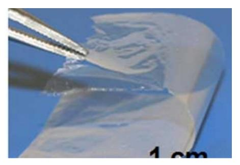
Could a seemingly simple clear plastic bag—the kind that you load your fruits and vegetables into at the supermarket—actually be as strong as steel? It could be if it is made from a new composite plastic that blends the strength of nanoparticles with the pliancy of a water-soluble polymer.
