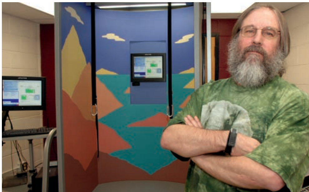
Robert Burkard uses this posturography booth, with painted horizon and tiltable floor, to study the causes of falls and the body’s reactions to stumbling. Photo: Nancy J. Parisi
